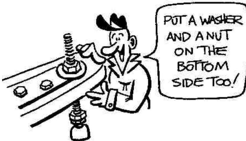
Install a hinge onto the tower as shown. Use glue and (4) 5/16"x1-1/4" bolts, washers and nuts.
