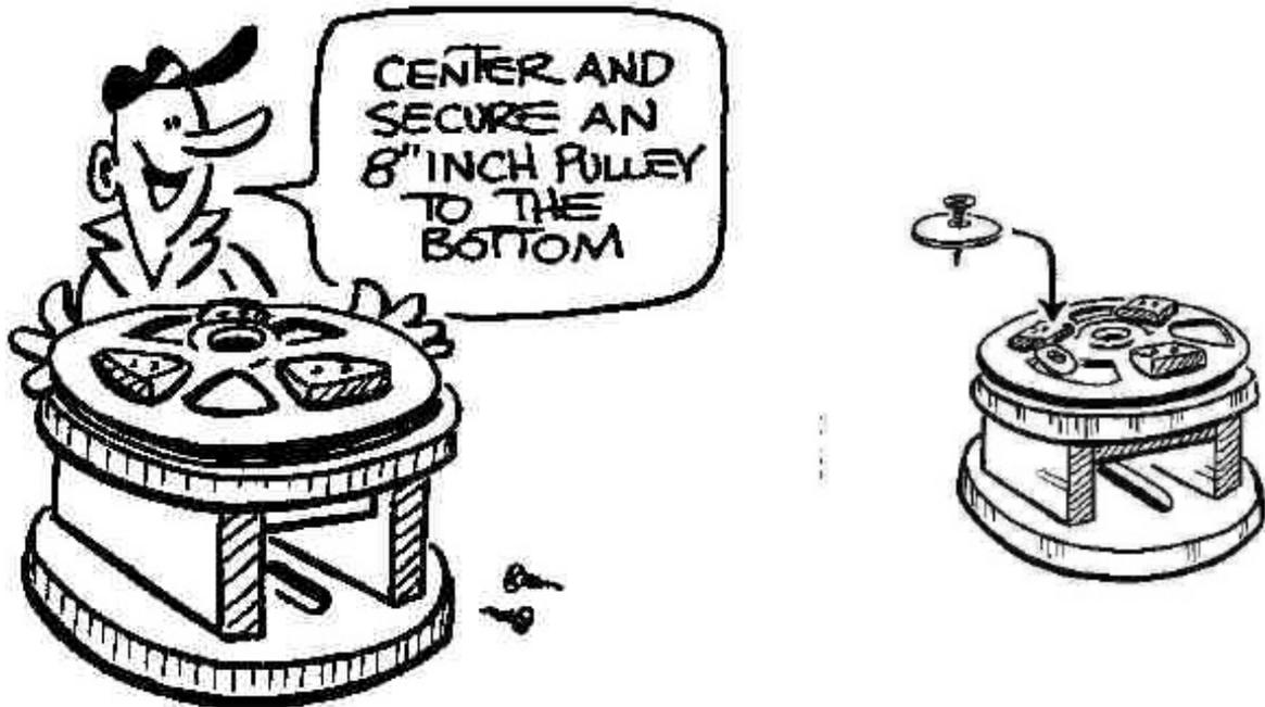
Cut three plywood dogs and attach them to the bottom of the eccentric in the same manner as the main platter. I also ran a screw and washer into the dog next to one of the pulley webs to avoid rocking of the eccentric. It is under some stress when polishing.
