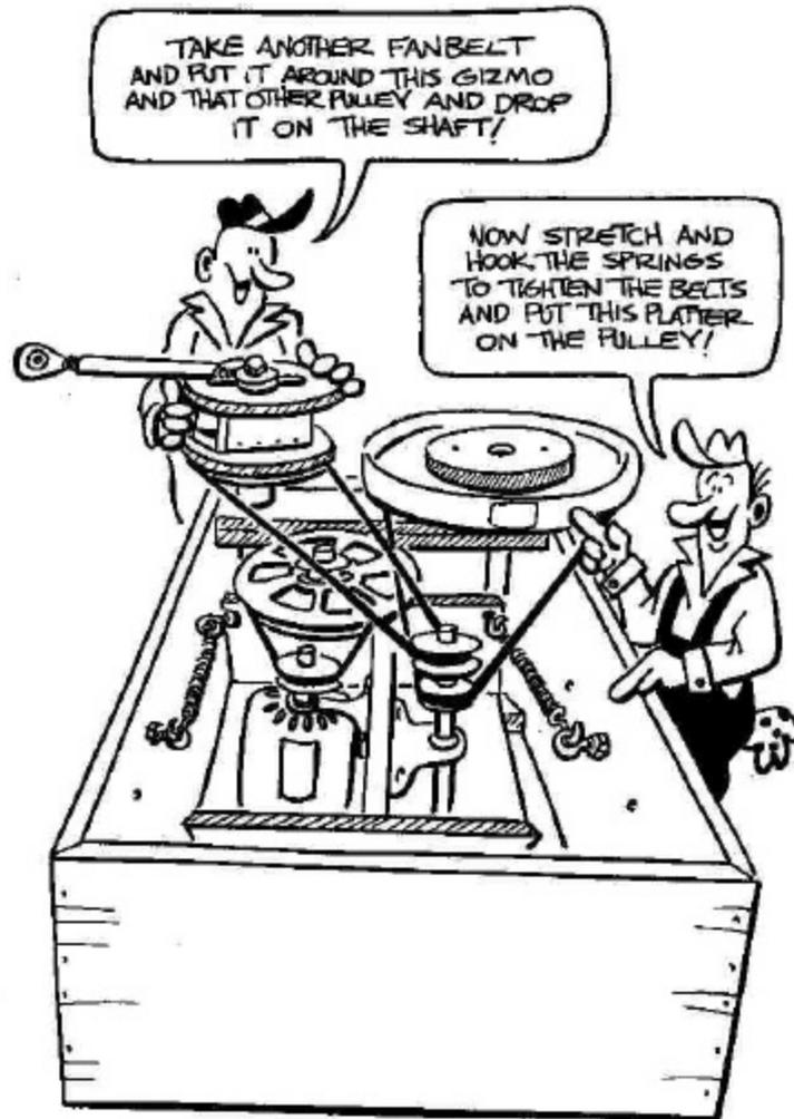
Install the eccentric and pulley combination as shown. Do not set the allen head in the 8" pulley.
