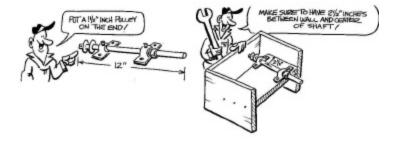
Use a 1/4 hp clockwise turning motorwith a **type 48 or 56** frame. This frame has slotted holes in it's base which are used to tighten the drive belt between the 1-1/2" motor pulley and the 10" intermediate drive shaft pulley.
