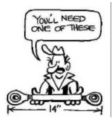
The eccentric drive rod can be made with either male or female rod end bearings.
