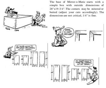
There is a fair amount of torque passing through the box, so be sure to glue all joints. I prefer using polyurethane glue. It is very viscous and swells slightly as it sets so small gaps will be filled. Align parts carefully. Once it sets, you will not be able to break the joints. Read the instructions for humidity requirements. Someglues require that the wood be dampened.
