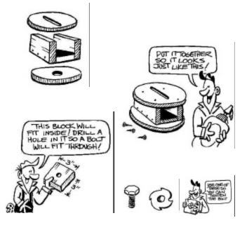
Drill a hole as required in the center of the  $3^{"}x3^{"}$ block. A  $3/8^{"}$  threaded insert (3 prong T-nut) needs to be pressed into it. This block will rest in the "tunnel" of the eccentric and catch the bolt that goes through the rod end bearing of the eccentric drive rod.
