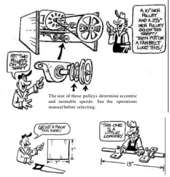
Cut the 7"x7"low speed shaft mount from a piece of plywood. You will also need a 5/8"x13" shaft and two bearing sets.
