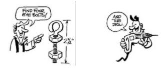
Drill holes into the sides of the base box as shown for the spring eyehooks. Thesewill be used to tension the drive belts from the powerhead. By moving the hooks, the powerhead can always be in a position to tension both belts.
