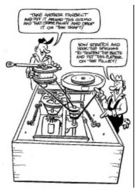
Install the eccentric and pulley combination as shown. Do not set the allen head in the 8" pulley.
