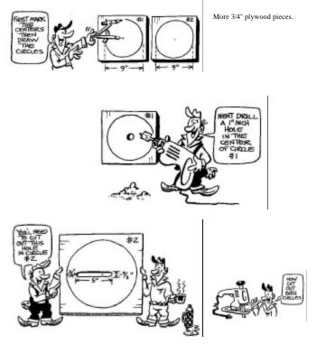
Note: Theslot can be made 4 inches long and stopped at the center of the circle. This will make finding the zero eccentric location easier.
