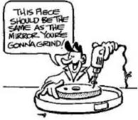
Build a hat section of 3/4" plywood the same diameter as the mirror or tool that will be attached to the turntable.
