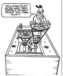
If you have not yet done it, install a 3/4" collar and thrust washer on the turntable and eccentric shaft. This will keep the pulley from contacting the plywood base. The eccentric collar should be 1" higher than the turntable collar. Now install a 12" pulley on the turntable shaft. Make sure that the pulley heights are correct and that the belts run true. **Do not** set the allen head in the pulleys. Throwit away. The aluminumpulley runs directly on the shaft. Use a little oil or grease.
