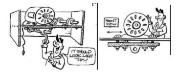
Mount the 7"x7" base onto the 2-1/2" motor bolts. Make sure that the base slides on the long bolts. Add 5/16" washers and nuts to the long bolts and tighten just barely snug.
