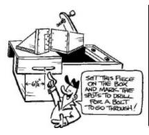
Set the entire overarm assembly on the base box and mark and drill the holes that secure them to each other. A 5/16" threaded insert needs to be installed inside the box to catch the 5/16" x2" bolt and washer that holds the pieces together.
