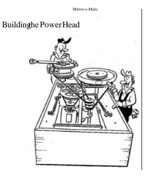
The heart of Mirror-o-Matic is the power head assembly. A single speed 1725 rpm1/4 horsepower motor is used along with a pair of belt reduction shafts and pulleys.
