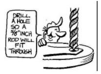
I used a piece of 5/8" threaded rod as the pin that will fit into the mirroror tool. The swivel (also called a toggle or leveling pad) is threaded for a 5/8"x11tpi rod. A 5/8" jam nut will keep the swivel from working loose.
