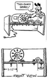
Install a 1-1/2" motor pulley on the end of the motor shaft. Tighten the set screw.
